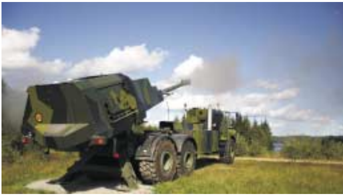
Potential Protected SP Howitzer - BAE Systems Bofors Defence 'Archer' currently undergoing joint trials with the Swedish and Danish Defence Forces.
