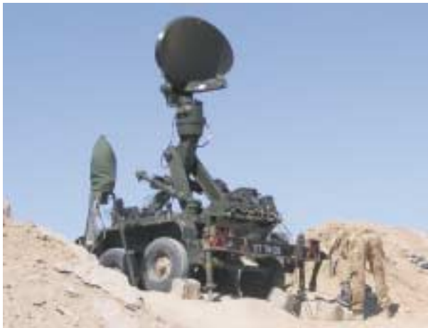
Ground Data Terminal. Line of Sight is critical. Not a major problem in Iraq but consideration to future theatres will dictate different deployment requirements.
