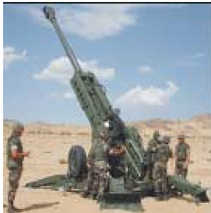
Potential Lightweight 155mm Towed Howitzer - M777 introduced into service in the USA in 2005 and Canada in 2006.
