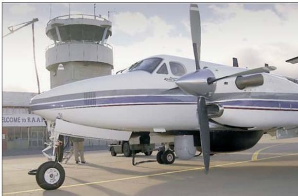
Figure 4: Project Ingara SAR installed on 173 General Support Squadron King Air
