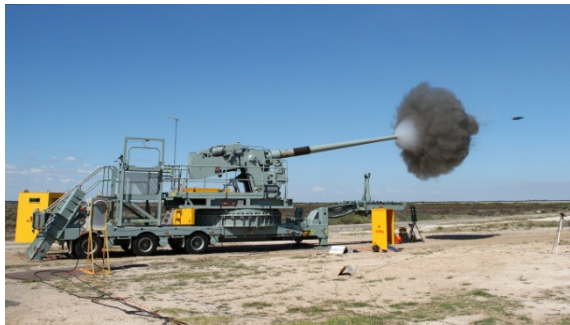
Figure 3 - 5/54 Mobile Proof Gun Mount – primarily used for in-service-surveillance of propellant.
