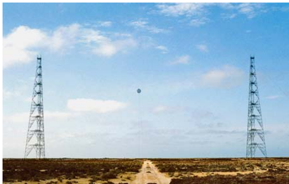
Figure 1 - Variable Time Towers for testing of proximity fuzes. The suspended metal ball will trigger fuze operation as the projectile passes close by.
